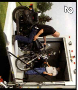
2 Raise lift gate using the hand held control
